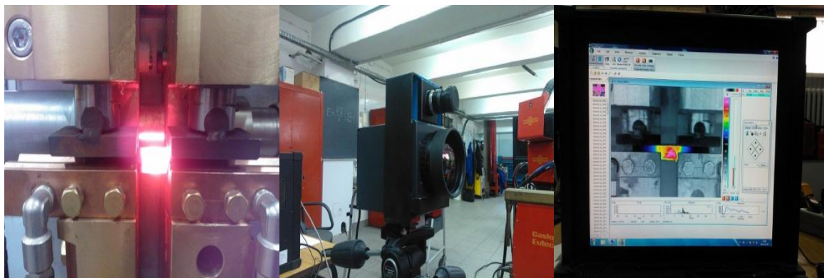
Figure 1. The testing setup for the simulation and recording of welding thermal cycles, 1-resistive welder, 2 - thermal imager, 3 - a computer
